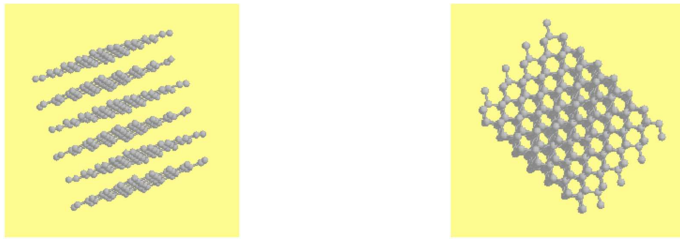
FIG. 1: On the left, the graphite lattice has a preferred slicing, contrary to the diamond lattice on the right [16].
