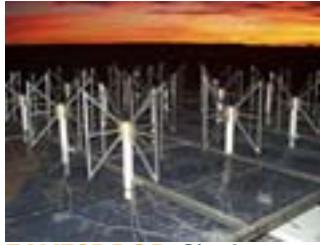
EAVESDROP Single antenna tile from the Mileura Wide-Field Array. Image Credit: Frank Briggs (Mt. Stromlo Observatory)
